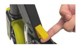
(2) Loosen the aluminum quick release, pull up the yellow folding handle, unfold the e scooter, then fasten the quick release on the folding mechanism.
