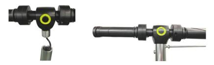
(4) Insert the cable and scooter head into the upper stretchable tube, fasten the scooter head with two screws, then fasten quick release on the pole.
