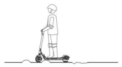
(12) Keep your speed between 4.5 - 9 km/h when you ride through speed bumps, elevator door sills, bumpy roads, or other uneven surfaces. Slightly bend your knee to adjust the balance.
